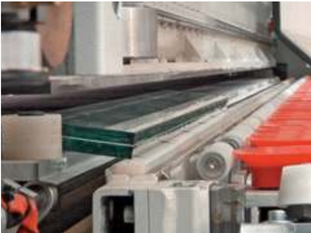
Cutting + breaking + standard removal, 60 mm.
