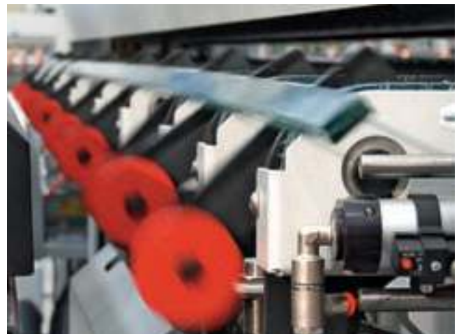
Cutting + automatic breaking + manual removal, 20 mm.
