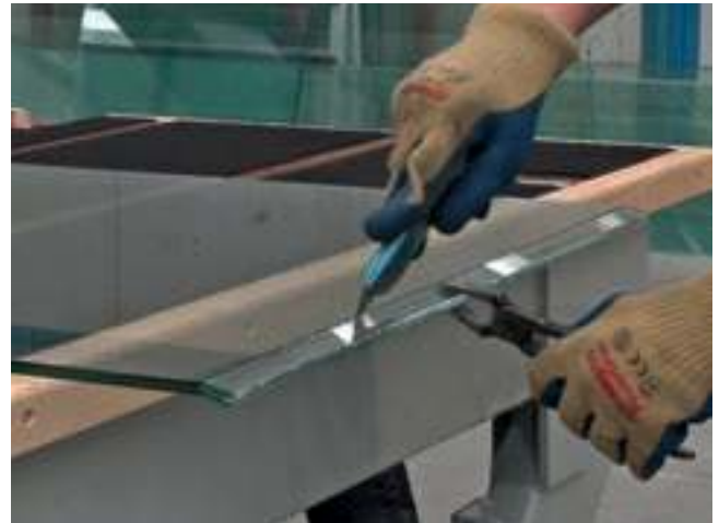
Cutting + automatic breaking + manual removal, 20 mm.
