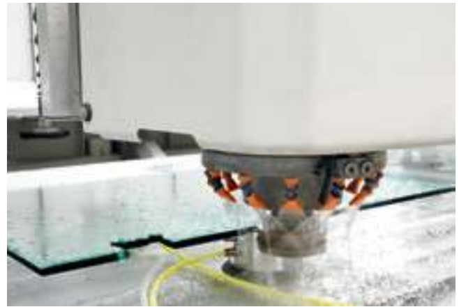
Peripheral grinding of the cutting edge.
