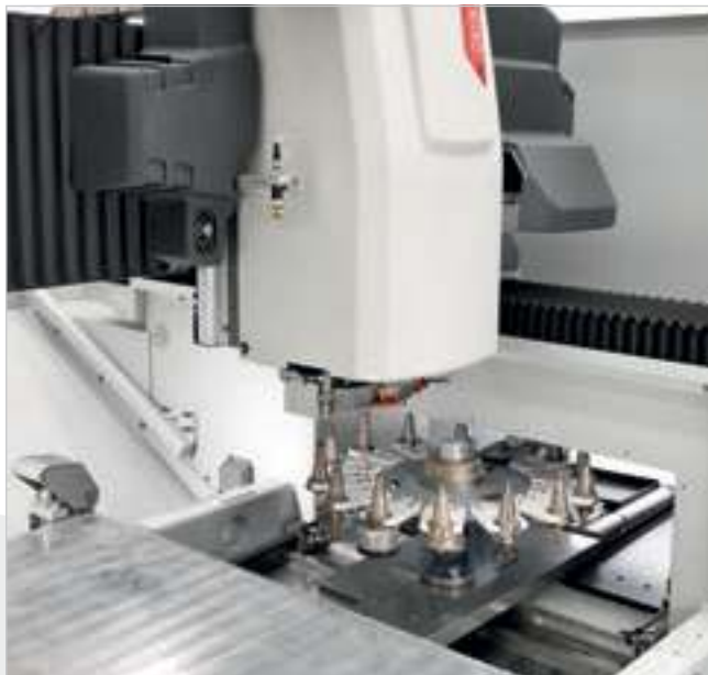
Rotary tool magazine on which the tools can be safely loaded even while the machine is working.
