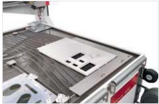
Aluminium square for panel positioning.
