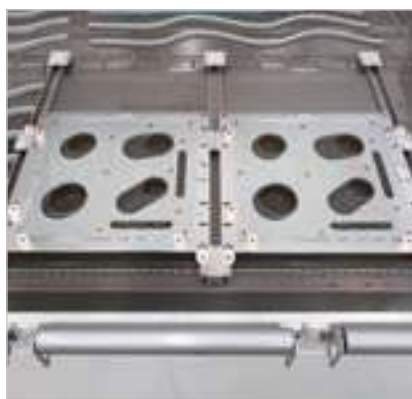
Option of placing more than one template on the work table, in order to increase productivity.
